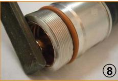
Remove PVC tape. File outer conductor flat with the outside of the connector mating surface. Remove any debris from the back nut. Apply silicone grease to O-ring. Place Oring in position on back nut.
