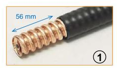
Straighten the cable for at least 300mm and ensure that it is cut square. Cut the jacket 56 mm from the end of the cable. Remove "Polyment" using white spirits, cloth and scouring pad until copper is clean. Deburr the end of the outer conductor. Burrs and sharp edges may damage the silicon gasket and its ability to correctly seal when fitted in the nex step.
