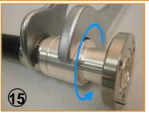
Tighten the connector body onto the back nut using a 36mm torque wrench whilst holding the back nut still with a 32 mm spanner. Torque to 50 Nm.
