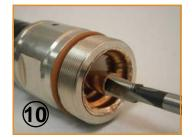
Thread inner to a min. depth of 15 mm using M8x0.75 roll-form tap. Remove any swarf and ensure all components are totally clean prior to final assembly.
