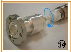
Screw connector body clockwise onto back nut, keeping the cable and back nut stationary.
