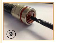
Verify the internal diameter of the cable inner. If the diameter is less than 7.6mm, widen the diameter with a 7.6mm drill bit for at least 15mm deepness.
